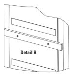
3. Fit the enclosure into the wall. The bottom edge of the bottom L-brackets will rest against the baseboard two-by-four. At this time, make note of adjustments necessary to square the enclosure into the wall (see Detail C).
